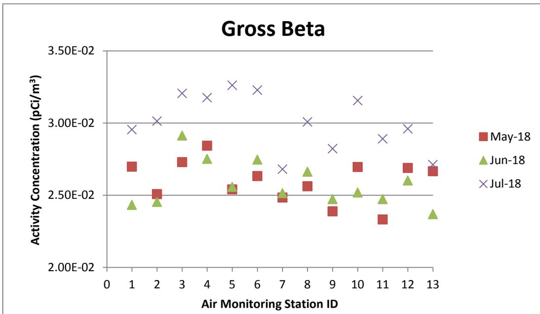
**Figure 9 Graphical Representation of Gross Beta Results in pCi/m<sup>3</sup>**
