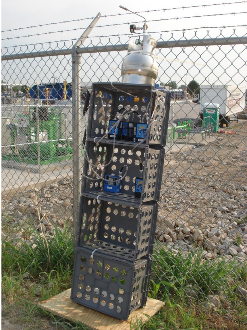
Figure 10 Ambient air sample collection structures and pump assemblies
