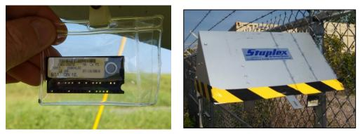
Mirion Technologies forwards 16 new TLDs to the Site approximately 5-7 days prior to the quarterly change-out event. The 16 TLDs include 13 for each sampler, a duplicate TLD for one of the samplers (the location is rotated), a field (control) blank, and a trip blank. Upon arrival, the packages are examined to verify the number and designations of the new TLDs.
