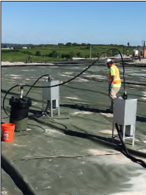
Photo #3 High volume sampling of source gas from under the EVOH.
