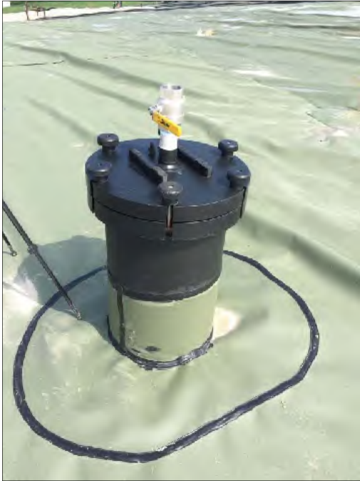
Photo #1 Source Gas Sampling Flux-box.
