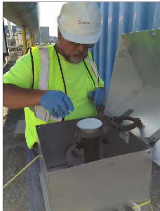
Photo #8 Setup of Ambient Flare Dioxin Sample.
