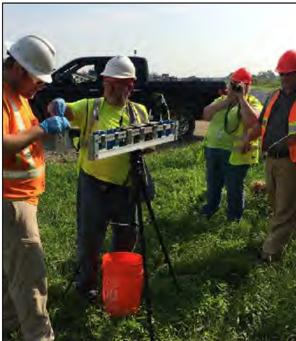
Photo #7 Setup of Ambient Sample Pumps with MDNR oversight.
