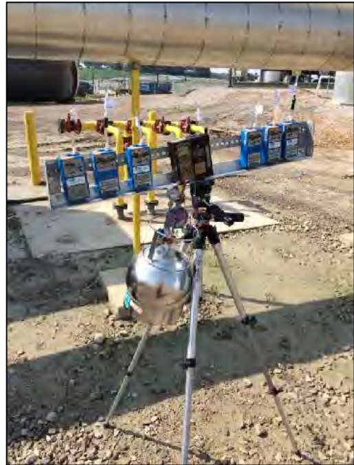
Photo #6 Ambient Sample Pumps Setup at Flare Station.
