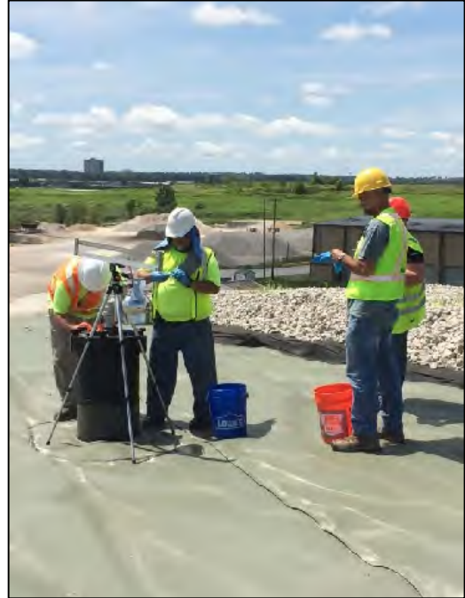
Photo #2 Collection of samples from the sampling port on the flux-box.
