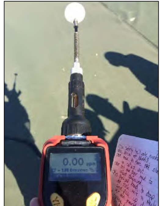
Photo #4 Benzene monitoring of High volume source gas exhaust at the south quarry location.
